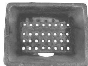
Example of clean grate
